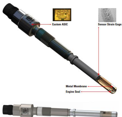
Figure 1: Sensata's Cylinder Pressure Only Sensors (CPOS)
