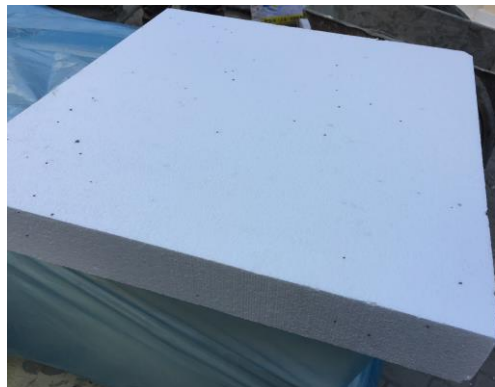
Figure 5. Polystyrene material used by GBT to be installed into existing buildings.
