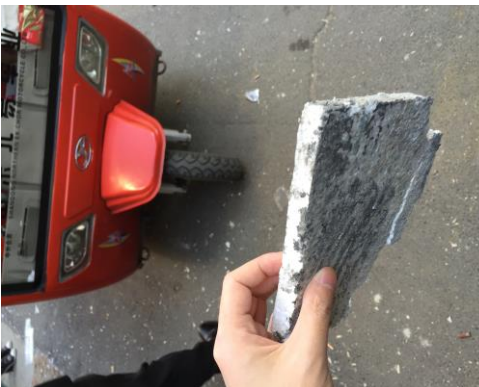
Figure 4. Polystyrene material used in existing building walls.
